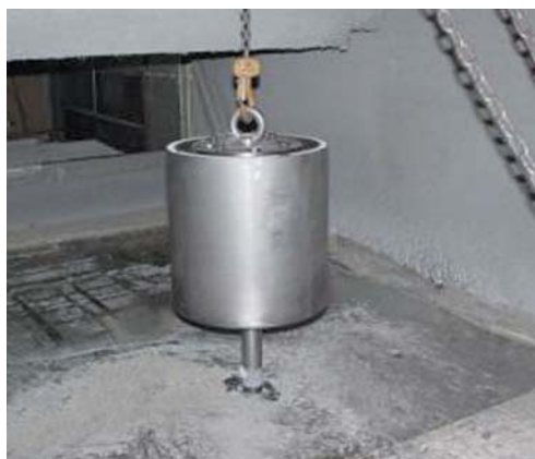
Lifma collecting iron powder from molten aluminum at 650°C
